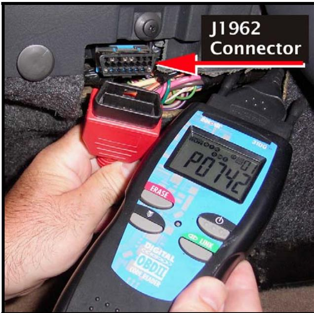
Figure 3: OBDII Scan Tool
