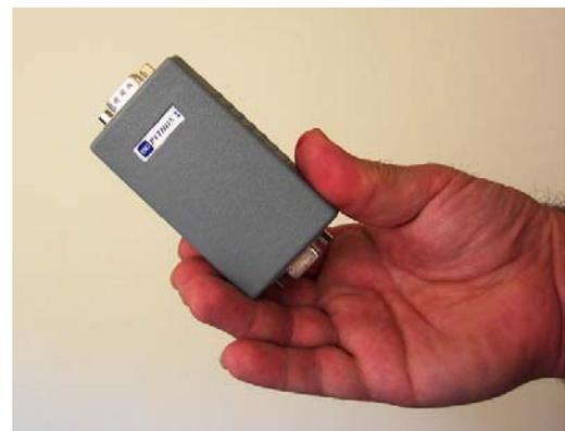
**Figure 7: J2534 Pass Through Adapter**
