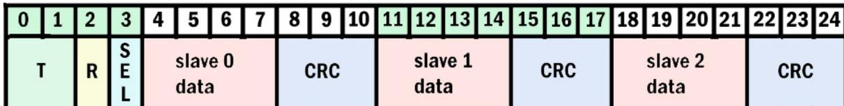
Figure 7 (copy) S-Frame with 3 Sensors and 4 bit Data
