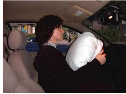
**Figure 10 Correct Driver Airbag Deployment**
