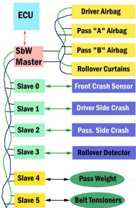
Figure 1 Example Safe-by-Wire Network
