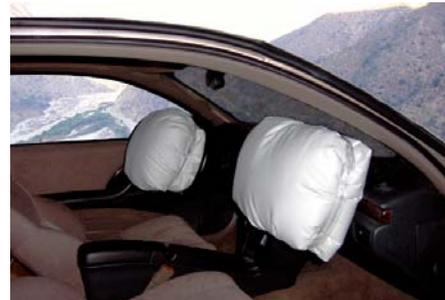
**Figure 11 Front Airbags Deployed**
