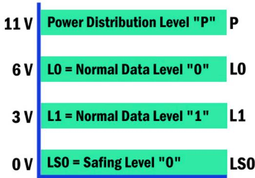
**Figure 3 Differential Bus Voltage States**
