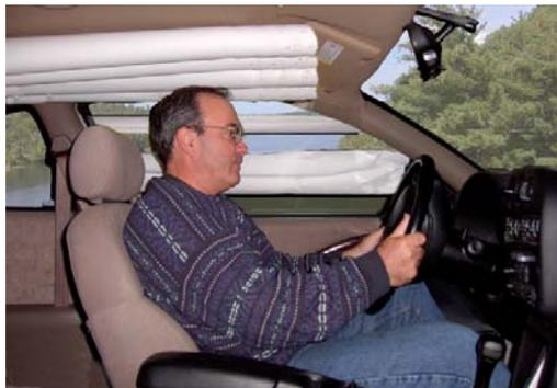
**Figure 16 Curtain Airbag with Roof Airbag**
