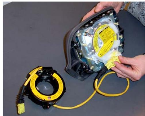
Figure 2 Steering Column Driver Airbag Module
